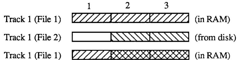
Use the dial to select the desired file, then type in the measure number. Data from the selected file will be added to the current tracks at the selected measures. The current song (with the additional data) may then be saved to disk.
