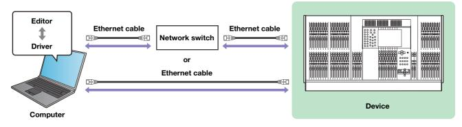
When you connect the computer to the M7CL directly, use a crossover cable.
