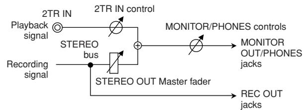
**NOTE** If the input channel PFL switch is on (■), then only the PFL output from that channel is sent to the MONITOR OUT jacks, PHONES jack, and level meter.
