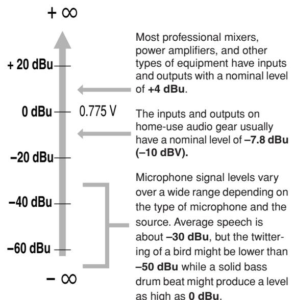
Most professional mixers, power amplifiers, and other types of equipment have inputs and outputs with a nominal level of **+4 dBu**.
