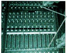
Panel plate パネルプレート 3. Insert plier tips into the front edge of the module ① and hold and lift up the right side of the part ① with the pliers. (If you try to insert the pliers in the opposite direction, the left side of the part ① cannot be lifted.) Support the module with your other hand so that you will not drop it if the plier slips. Be carefulnot to pinch your fingers.
