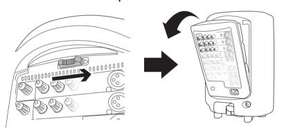
Open the cover panel attached to the other speaker, and then remove the box from inside the accessory compartment.
