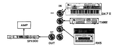
With these connections, pressing the SELECT key on the PLS1 panel allows you to select the signals to be input to the SPX900 in sequence.
