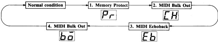
In Utility mode, the LED on the <u>UTILITY</u> key lights to indicate it is in use. In this condition, patching patterns cannot be stored or recalled.
