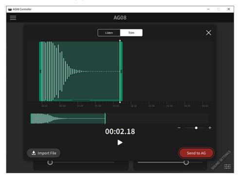
Press the [Import File] button to select an audio file and import the data into the AG08 Controller app. Use the onscreen controls to adjust the length of the audio file, and press the [Send to AG] button to send the data to the AG08. You can adjust the length and trim (delete) the silence at the beginning and end of the recorded data, both for audio files saved on your computer or iPad and for data saved on the AG08.
