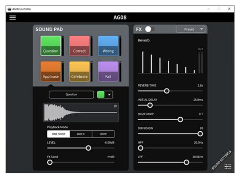
Select the pad to configure in the top left part of the screen. Set the parameters in the bottom left part of the screen for the pad you selected, including the name (Rename), the pad's LED color, waveform display, playback mode, pad output level and FX send level.
