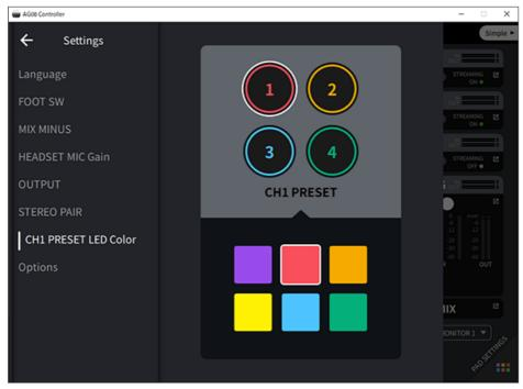
• When channels 1 and 2 are linked as a STEREO PAIR (p.70), presets cannot be registered and the preset buttons go dark.
