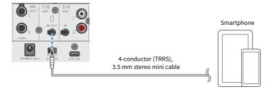
The default output setting for the smartphone input/output connector is AUX, which prevents the other party's own voice from looping back to them when you are making a smartphone call.
