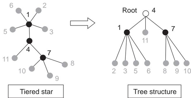
The above diagrams show the frequently-used tiered star (multiple stars that are connected) as a tree structure. In a tree structure, nodes that are not connected to another node in the direction away from the root are called **“leaf nodes.”** In the above diagrams, these nodes are shown in gray.
